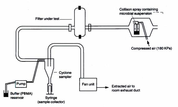
For the filters tested at 55 litres per minute a May Bottom Stage air sampler was used instead of the cyclone sampler.
